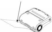
(5) To discharge the paper from the printer, hold down the FEED switch.
